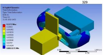
Fig 11: Simulation graphic of Low Speed Impact Test
